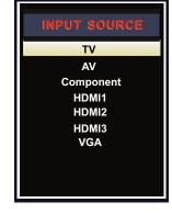
Press **INPUT** button on the TV set or remote control to display the input source menu, and use **CH+/-** button on the TV set or  $\land$  /  $\lor$  button on remote control to select the input source, press **OK** button on the remote control to enter.
